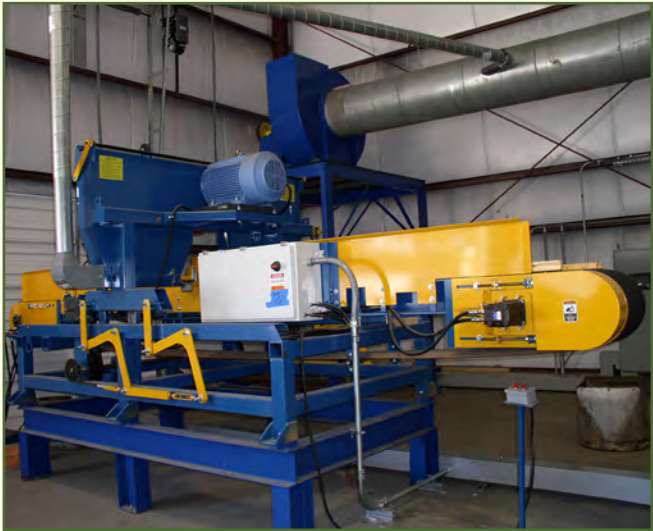
Baker “D” model resaw with 16” x 16” capacity: Allows for larger capacity using 1¼” or 1½” blades with heads on both of the conveyors so boards are cut on each pass, minimizing down time and the time needed to return uncut material.
