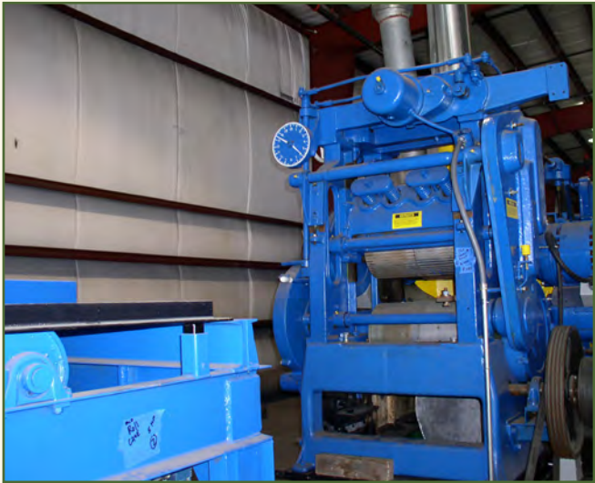
Stetson-Ross Timber Sizer with 16” x 24” capacity: Accurately sizes finished timbers to within 1/16 of an inch by planing all four sides of a timber up to 16” x 24” x any length in a single pass.
